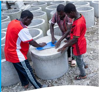
Toilet rims and slabs fitted with SATO pans. Toilet business owners (TBOs) are innovating and building smart toilets that are easy to install. TBO, Lukman Abubakar now makes concrete rims and slabs fitted with SATO pans used for making smart toilets in Tilden Fulani, Toro LGA Bauchi state, Nigeria.
